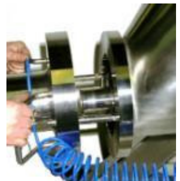
Dismountable end shaft bearing mixing screw Extraction mixing screw: by pulling it out
